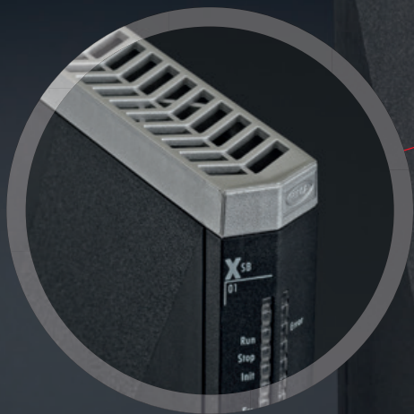
Front panel and ventilation caps – pushed on and locked in place
